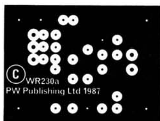
Fig. 3: Full size double sided track pattern and component layout for probe p.c.b.
