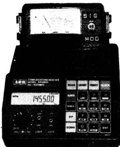
Installed modulation and signal meter showing suggested calibration
